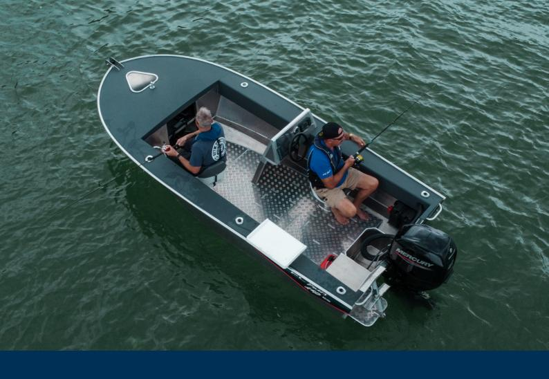
Every FC boat including the FC 390ss comes with a built in "FC Passive Live Bait Tank to target bigger fish as well as the FC Dry Riding Gunnel System which keeps you dryer and more comfortable. Safety is catered for with positive buoyancy in both the fully-welded tread plate floor cavity and the closed cell foam-filled gunnels.
