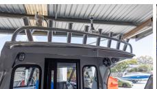
**FULLY WELDED ROD HOLDERS**
